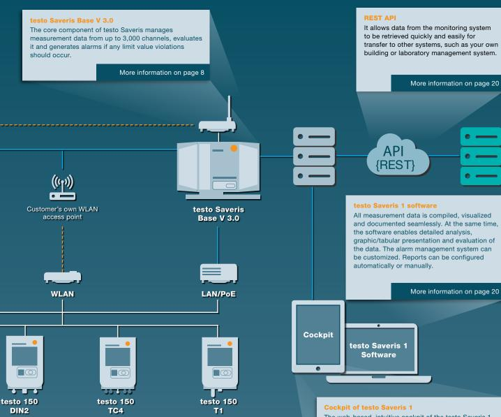
The web-based, intuitive cockpit of the testo Saveris 1 software makes it possible to detect alarms at any time, to initiate corrective measures and to acknowledge them. Alarms are clearly displayed in the cockpit. Each acknowledgement of an alarm must be completed with a personalized, digital signature as well as a mandatory comment on the event.
