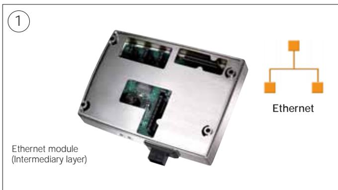
The Ethernet module is an intermediary layer („sandwich“ design), which can be optionally integrated into the transmitters testo 6681/6351 ex-works. It can also be subsequently easily and quickly retrofitted on site. Two LEDs provide the responsible system operator with information on the status of the voltage supply and the LAN connection.
