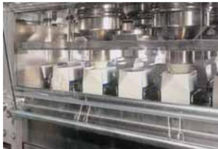
Positive pressure in the filling room maintains the hygiene conditions during filling operations in the food and pharmaceuticals industry
