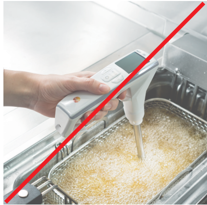
Figure 30: Wrong – measurement with product being deep fried
