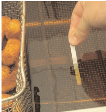
Figure 22: Measuring free fatty acids using a test rod
